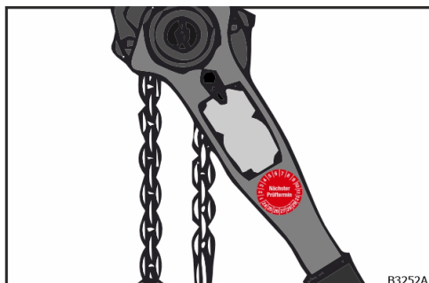
Fig. 49: inspection sticker (lever chain hoist)
