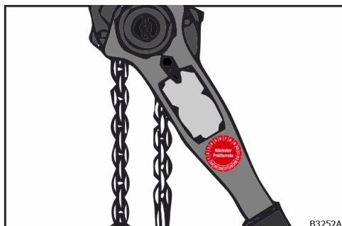
Fig. 106: inspection sticker (lever chain hoist)
